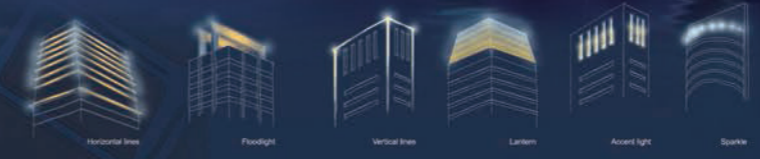
Building Crown Lighting Methods
